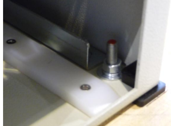
Figure 1: Showing the two different locations of the bolts that hold down the BTRSD for shipping
