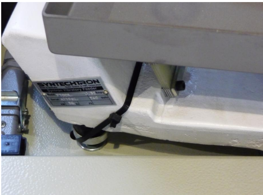
Figure 2: Showing the black strap securing the vibratory feeder for shipping
